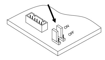
When programming is completed, move the mini jumpers to the **OFF** position.
